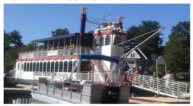
Two Paddle Wheels alternated direction of rotation and application of power in ordered to maneuver us away from the dock and make the boat turn to get the stern in the right orientation before set off for the lake from the cove mooring.
