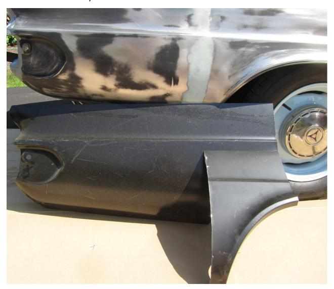
In the above picture note the FLRQRP was installed as received without any modifications but the rear panel had to be cut to match the FLRQRP. The cutoff can be seen in the picture.
