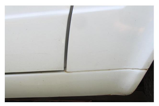
The above show the rust creep starting along the seam. The following picture occurs when the FLRQRP is installed with the vertical seam virtually eliminating the horizonal rocker seam:
