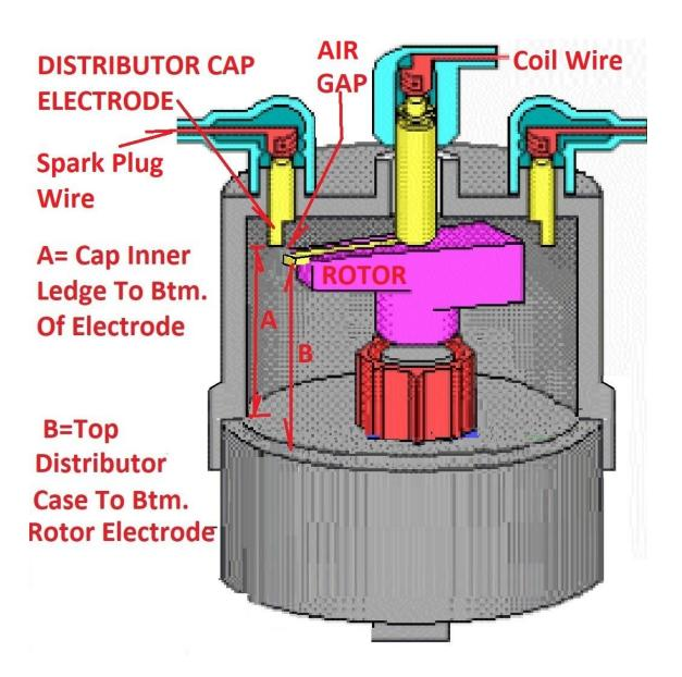
Part 1 cap measurements focused on comparing the A and B dimension to determine the up/down gap that might be occurring because the cap was built with the distributor terminal too high up in the cap. Said another way the rotor wasn't reaching up to the distributor terminal far enough. Part 2 concerns the diameter of the distributor terminal itself.
