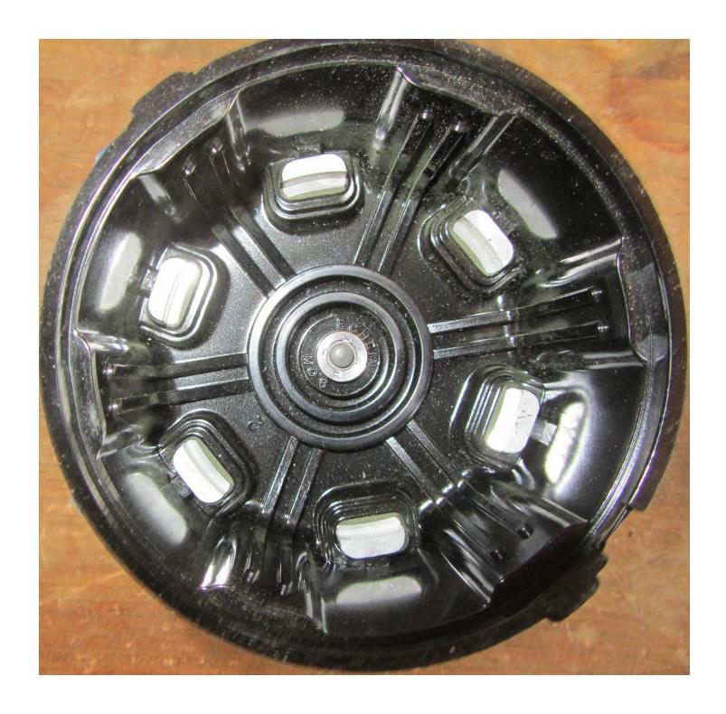
Bottom Line: Measure the diameter of the distributor cap terminals while standing in the store. Expect numbers to range from 3/8 down to an itty bitty 5/32. Grab the cap with the biggest terminal diameter you can get (& meets the up/down measurement criteria).
