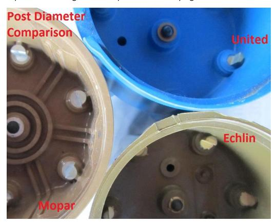
It's obvious that if the terminal needs machining there is little material to machine on the United cap and more on the Mopar cap. But more importantly these diameters effect the side to side air gap between the rotor and distributor cap terminal.
