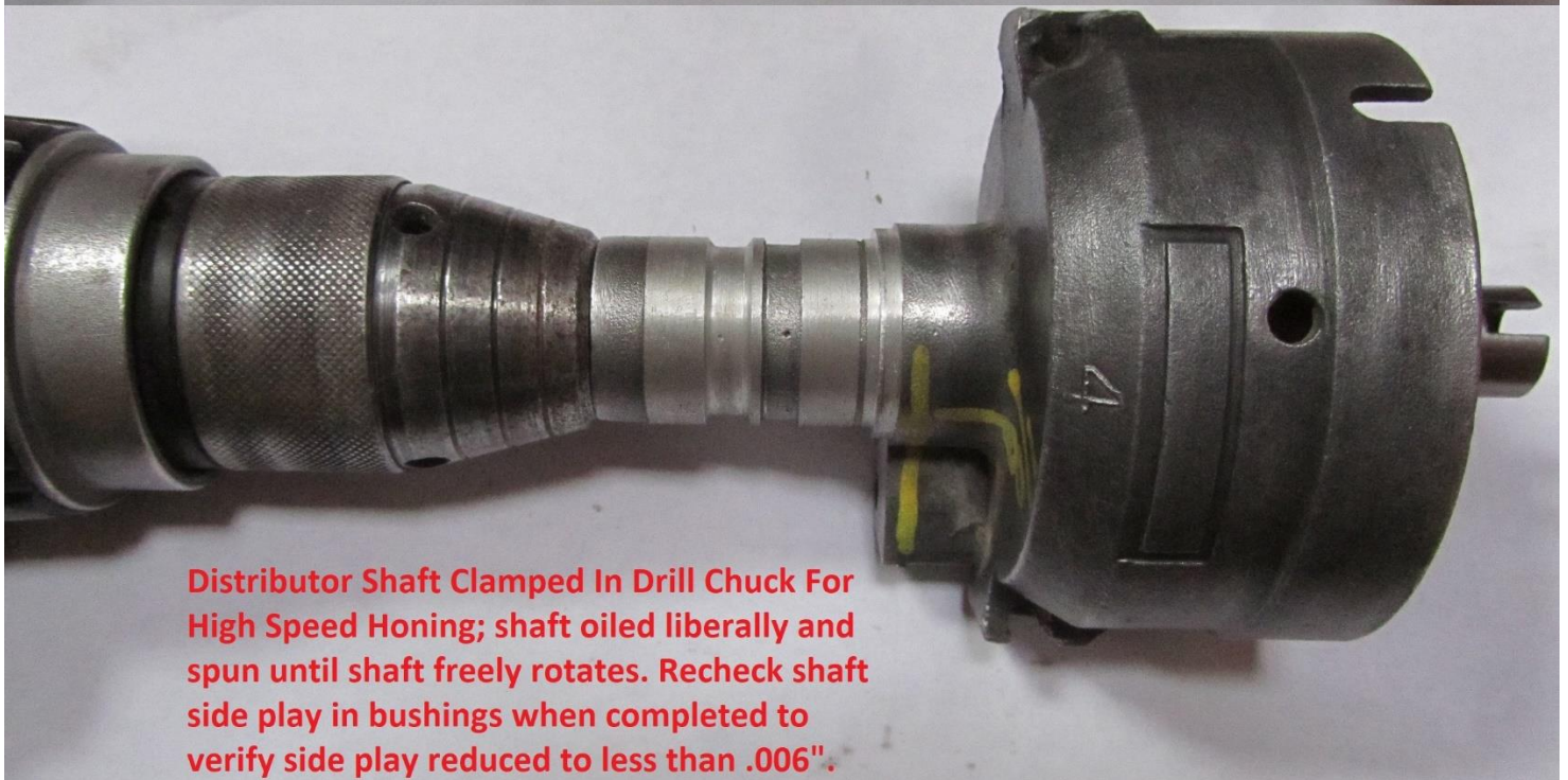
1/2" Drill Chuck Opened Full Amount To Accept Distributor Shaft For Honing Bushings
