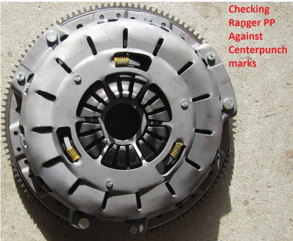
99 Ford Ranger 3.0L 9 1/8 Diaphragm Pressure Plate:
