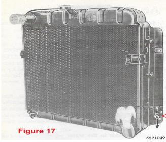
RADIATOR—To test for cloqged radiator core, remove the top and bottom radiator hose and insert plugs in the inlet and outlet connections. See Figure 17, Fill the radiator with water. Then remove the plug from the bottom connection. If the passageways in the core are not clogged, the column of escaping water should extend 5 to 6 inches above the lower connection.
