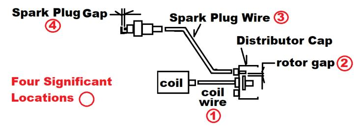
Part 2 will review the importance of inspecting Secondary voltages & causes. Why spend the time doing this? Excessive Secondary voltages can lead to component premature breakdowns such as the coil itself, ECU if present, Distributor Cap/Rotor/Point terminals, & Spark Plugs.
