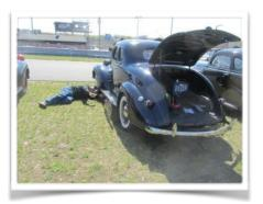
One Plymouth got some brake work while on the Field which including rodding out the master cylinder compensating port to relieve built up pressure in the brake line as well as some troubleshooting of the generator cutout relay that had the points sticking which caused the battery to discharge into the generator.
